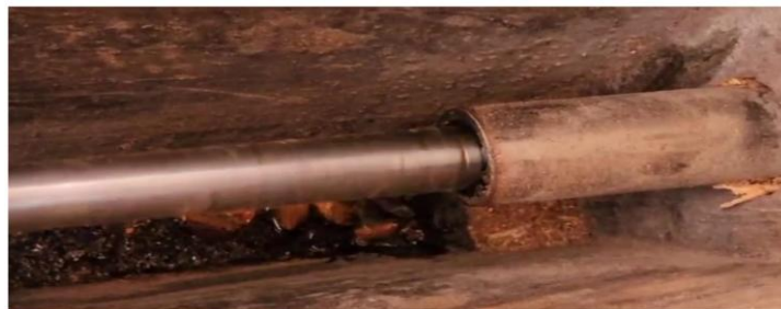
Gambar 4. Kendala air masuk melalui seal poros baling-baling.
